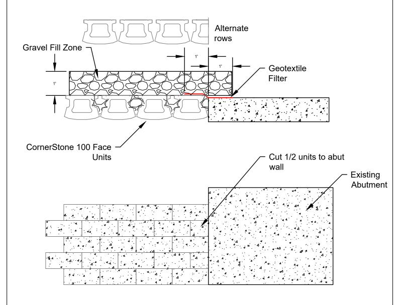
It is also a good practice to use bi-axial geogrid under the leveling pad near the area where the SRW abuts the exsting structure to minimize settlement.
